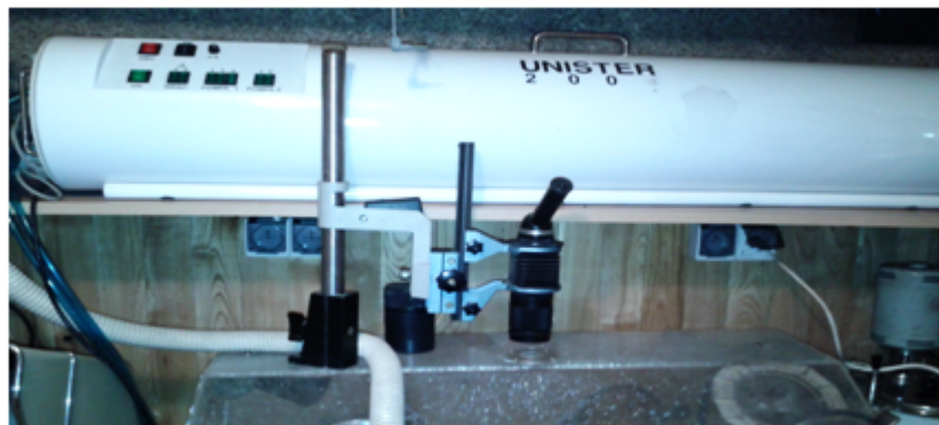
Fig. 2 Flow-through air and fluid sterilizer: (1) device diagram; (2) a prototype cooperating with a laboratory glove box, according to PL 164635
